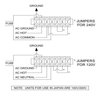
Fig. 3 Primary Power Wiring Diagram
