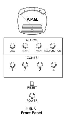
**Low Alarm Light/High Alarm Light:** The light is lit when the function is active.
