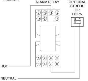
Fig. 4 Option Connection Wiring Diagram
